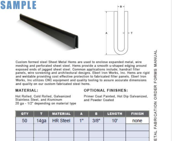
Hot Rolled, Cold Rolled, Galvanized Stainless Steel, and Aluminum 20 ga - 1/2" depending on material type Primer Coat Painted, Hot Dip Galvanized, and Powder Coated
