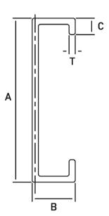
Bent Plate C-Channels are used for a variety of customer designed applications. Whether they're being used for girts, perlins, sub-girts, stair treads or building framing; custom formed channels offer a strong cost effective option. Eberl Iron Works, Inc utilizes CNC equipment and quality tooling to assure accurate dimensions and quality on our custom steel forms.
