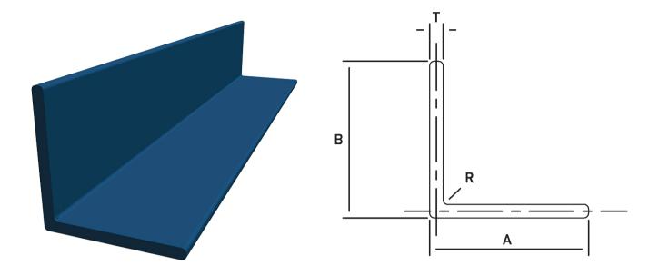
Bent Plate Angles are used for a variety of customer designed applications. Whether they're being used for concrete pour stop, lintels, corner guards, equipment framing or building enclosures; custom formed angles offer a strong cost effective option. Eberl Iron Works, Inc. utilizes CNC equipment and quality tooling to assure accurate dimensions and quality on our custom steel forms.
