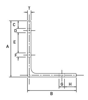
Bent Steel Plate Angle Clips are used for many connection applications Uses include curtain wall, concrete masonry and for structural steel connections. Eberl Iron Works, Inc. utilizes CNC equipment and quality tooling to assure accurate dimensions and quality on our custom steel forms.
